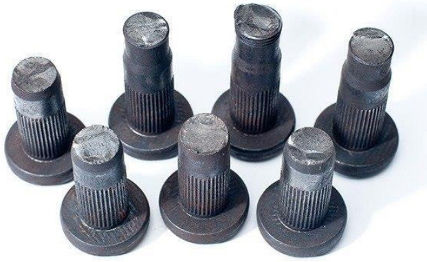
Fig No6: Fatigue fracture on Stud Figure indicates fracture on studs from a motor home. Right side wheel after 2900 miles.
